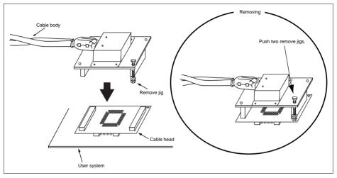
Figure 5 Fastening Cable Body
